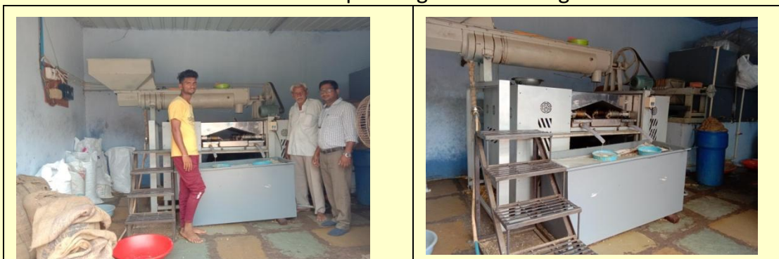
A view of cold press groundnut oil extraction unit with a capacity of 350 litres per day at Rulmaur, Yadgir district
